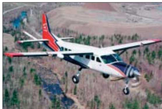
Figure 1 Cessna Grand Caravan fitted with an AIRGrav and magnetometer surveying system
