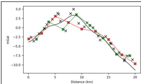
Figure 4: Original 500 m points (x's) with 2500 m sub-sampled profiles (red and green lines). 'Regional' gravity is the smoother black line.
