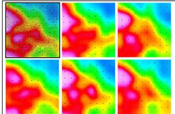
Figure 5: Original 500 m spaced survey (top left); 5 subsets using 2500 m spacing, offset from each other (other panels). A 5000 m full-wavelength filter has been applied.
