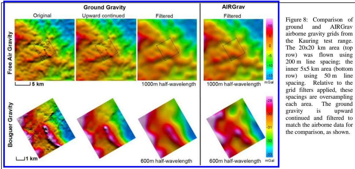
Figure 8: Comparison of ground and AIRGrav airborne gravity grids from the Kauring test range. The 20x20 km area (top row) was flown using 200 m line spacing; the inner 5x5 km area (bottom row) using 50 m line spacing. Relative to the grid filters applied, these spacings are oversampling each area. The ground gravity is upward continued and filtered to match the airborne data for the comparison, as shown.
