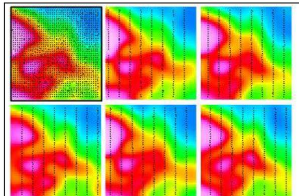
Figure 6: Original 500 m spaced survey (top left); 5 subsets sampling along 2500 m spaced N-S lines, offsets from each other (other panels). A 5000 m full-wavelength filter has been applied.
