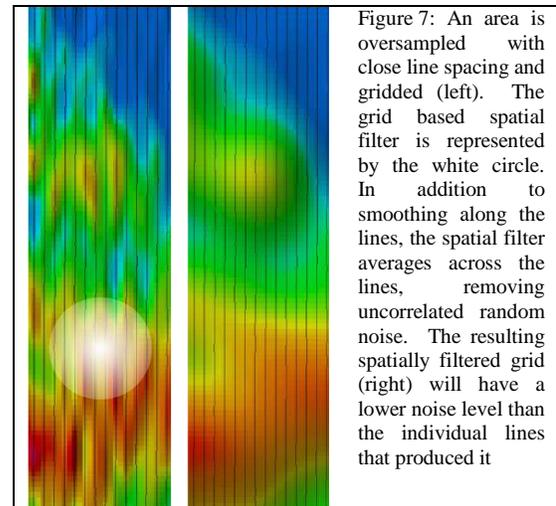
The Kauring test range again provides an example. The range was flown using an AIRGrav system in 2012 with 50 m line spacing in a central 5x5 km area and 200 m line spacing in the outer 20x20 km area (Sander Geophysics, 2012). Spatial filters of 600 m and 1000 m half-wavelength were used on gridded line data in each area respectively. Since these filters are larger than the 200 m line spacing, the area is oversampled relative to the filters
