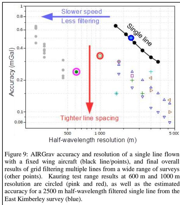
Figure 9: AIRGrav accuracy and resolution of a single line flown with a fixed wing aircraft (black line/points), and final overall results of grid filtering multiple lines from a wide range of surveys (other points). Kauring test range results at 600 m and 1000 m resolution are circled (pink and red), as well as the estimated accuracy for a 2500 m half-wavelength filtered single line from the East Kimberley survey (blue).
