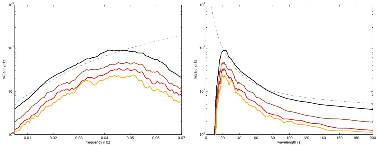
**Figure 8a and 8b** Noise spectrum for AIRGrav lines as a function of frequency (a) and wavelength (b). Curves are for individual lines (top curve) and groups of 4, 9, and 16 lines (progressively lighter red curves from top to bottom), achieving progressively lower noise level. Dashed black line is a theoretical GPS noise limit from van Kann (2004).
