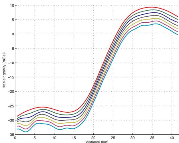
**Figure 4** The air truth filtered using a range of low pass filters from 70 s (light blue at bottom) to 170 s full-wavelength (red at top). Profiles are shifted vertically for clarity.
