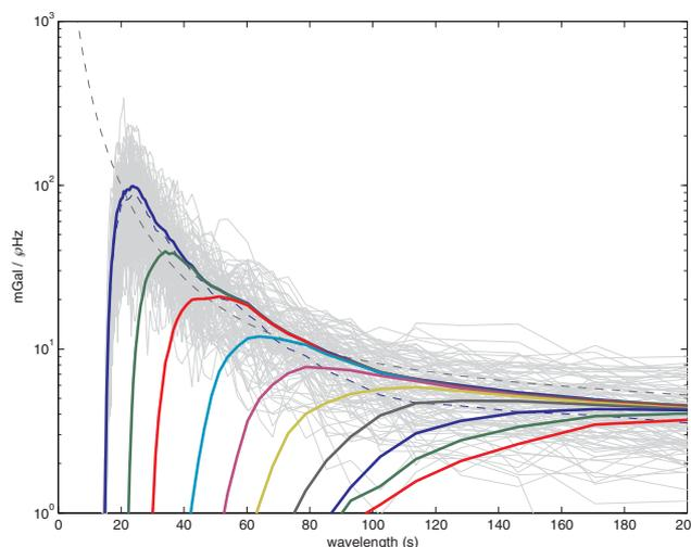
**Figure 6a and 6b** Noise spectrum for AIRGrav lines as a function of frequency (a) and wavelength (b). Different coloured lines are for different low pass filters ranging from 20 s mid-point (dark blue, highest amplitude) to 170 s mid-point (red, lowest amplitude). Grey lines are individual passes with the 20 s filter applied. Dashed black line is a theoretical GPS noise limit from van Kann (2004). Dashed blue line is the 20 s filter average spectrum when only the best 50 passes are used.
