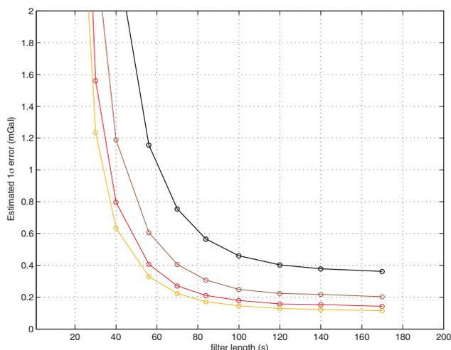
**Figure 7** Estimated accuracy of line data for the Ottawa repeat line for individual passes (top curve) and groups of 4, 9, and 16 passes averaged together (progressively lighter red curves from top to bottom).
