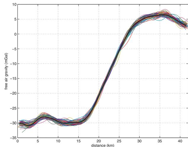
Figure 2 100 passes along the repeat line (coloured lines) and the average of all passes (heavy black line). A 100 second full-wavelength filter (0% pass at 75 seconds, 100% pass at 150 seconds) was used for this figure.
