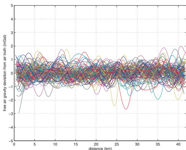
**Figure 3** Deviations from the average line for each of the 100 passes shown in Figure 2.
