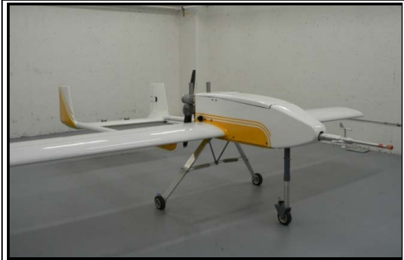
Figure 3: GeoSurv II prototype, March 2010 (without wingtip magnetometer housings).
