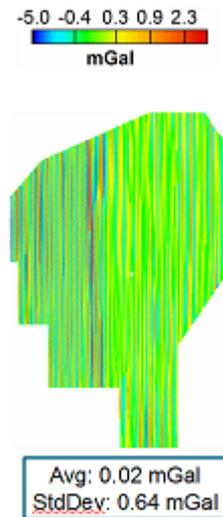
Figure 4. A grid of the leveling corrections applied to the Kimberley Basin survey data using the difference decorrelation method.
