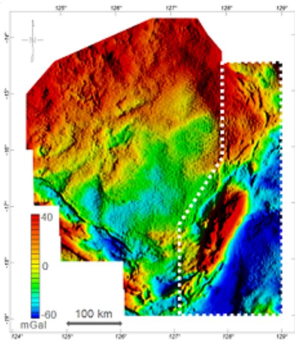
Figure 3. Airborne Bouguer gravity data of the Kimberley Basin Block levelled using difference decorrelation adjacent to Kimberley East Block data levelled with control lines (surrounded by the dashed line), low pass filtered (2.5 km half wavelength mid-point), with a sun shade from the east.
