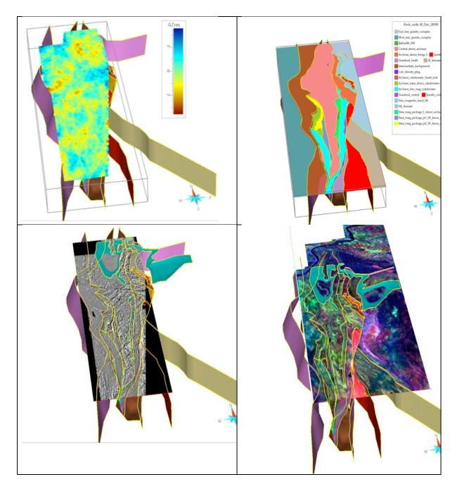
Figure 1. Curaçá Valley Region regional 3D integrated model representation. Top left: residual gravity overlain on modelled lithological domains; Top right: classifying different lithological compartments to assign physical properties for further modelling; bottom left, Total Magnetic Intensity (TMI) with lithological overlay, and (bottom right) lithological grouping overlaid on radiometric image to cross-check correct lithological classification.
