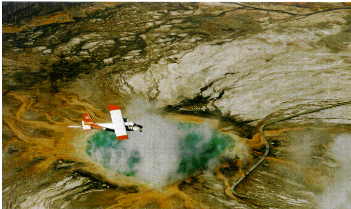
In most cases survey aircraft are required to fly low and slow in order to gather accurate data. The company's single Islander has the ability to fly constant speeds in mountainous terrain. In this case it was flying a survey over a geyser in Yellowstone National Park in the US.
