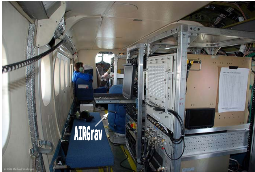
Photo of AIRGrav installed in the Kenn Borek DCH-6 Twin Otter ready for surveying. Photograph courtesy of Michael Studinger, Doherty Research Scientist for AGAP.
