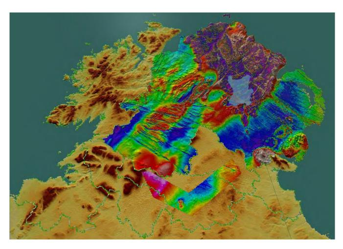
The airborne geophysics survey is an industry-standard low-level survey, comprising measurements of magnetic field, radiometrics and electrical conductivity. The line spacing will be 200 m and the flight direction 345 degrees, to correlate with existing surveys in the region.
